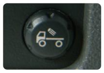
The cargo lamps provide illumination of the cargo area and the interiors of the top-box storage units. The controls are located near the exterior lamps control.
