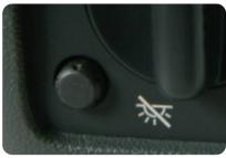
To prevent your vehicle's dome lamps from illuminating when a door is opened, press the dome lamp override button located below the exterior lamps knob.
