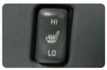
On equipped vehicles, the lower and back cushions of the driver and front passenger seats can be heated.
