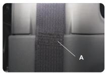
The safety belt shoulder straps feature a park stitch (A) to prevent the safety belt latch plate from contacting the interior trim panel when the safety belt is not in use. If you notice the latch plate contacting the trim panel, make sure the safety belt latch plate is located above the park stitch in the belt.
