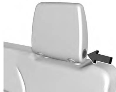
To fold the head restraint, press the button on the side of the head restraint.
