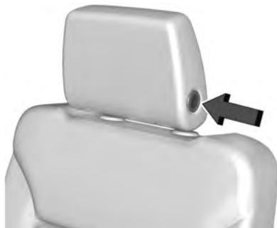
To fold the head restraint, press the button on the side of the head restraint.
